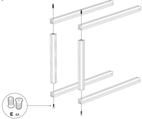
**STEP 02** Install the Standoffs on the Left Upper and Lower Side Brackets
